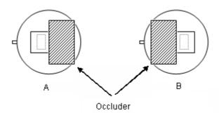
The sensitivity balance of dual element sensor is calculated through testing the sensitivity (single signal output voltage) of each element and using the following formula:
